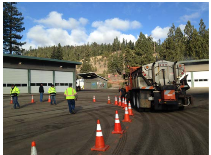
The project team set up cones representing the minimum inside center island diameter of the roundabouts and had the snow plow and street sweeper negotiate around the cones to ensure the size and shape of the proposed roundabouts is sufficient for maintenance operations. Photo by Hillary Isebrands.
